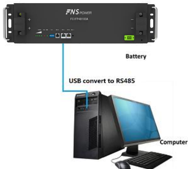
Figure 5-3: Communication Cable Connections between Battery and Computer
